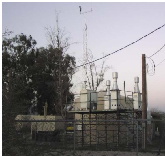
Rillito meteorological tower and particulate monitors on platform – 05/2010
