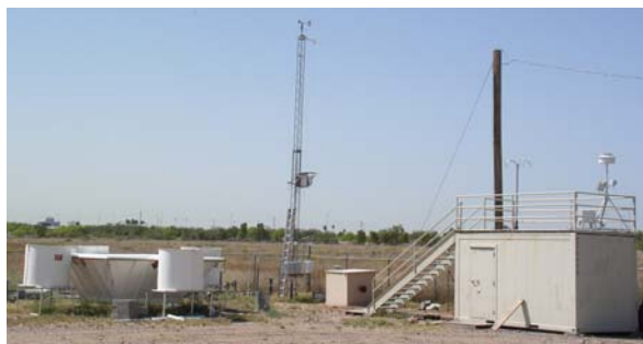
Wind profiler, meteorological tower, and shelter at VEL – 04/12/2005
