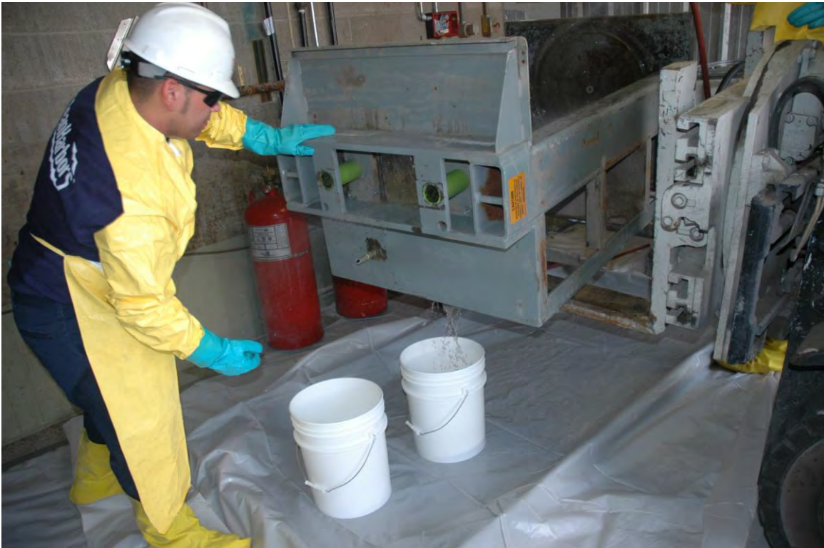
Photo #6: Collecting water samples from rinse process
