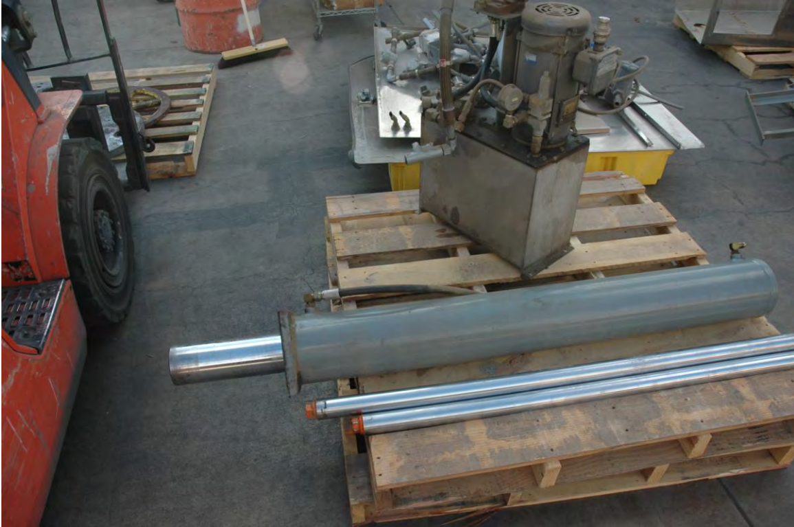
Photo #9: Hydraulic ram and pump assembly removed from unit
