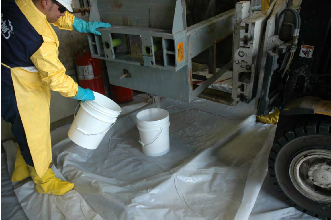
Photo #7: Collection of rinse water for rinse samples (second photo)
