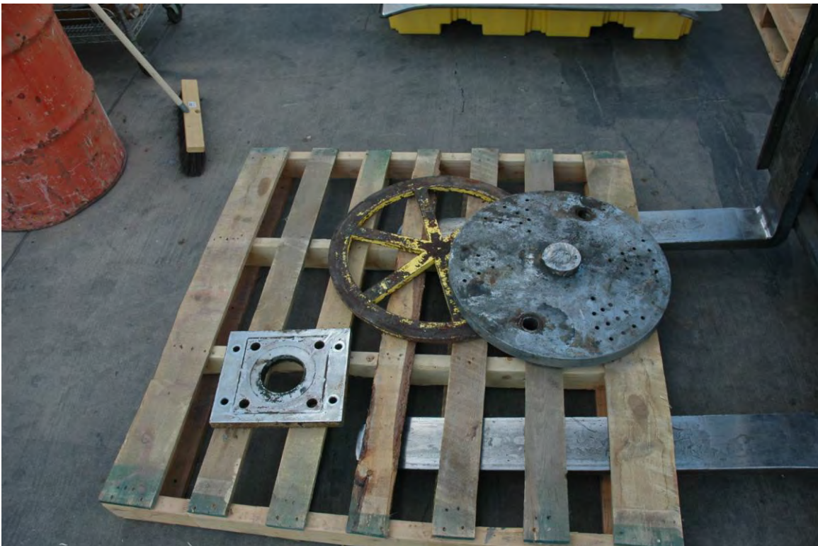
Photo #10: Plunger cut from hydraulic cylinder prior to cleaning
