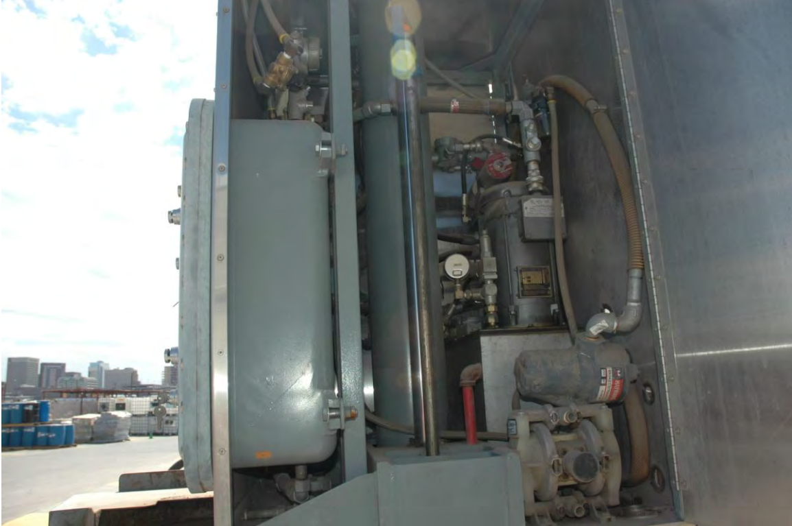
Photo #1: View into side door of 55 gallon drum crushing unit. Hydraulic system shown
