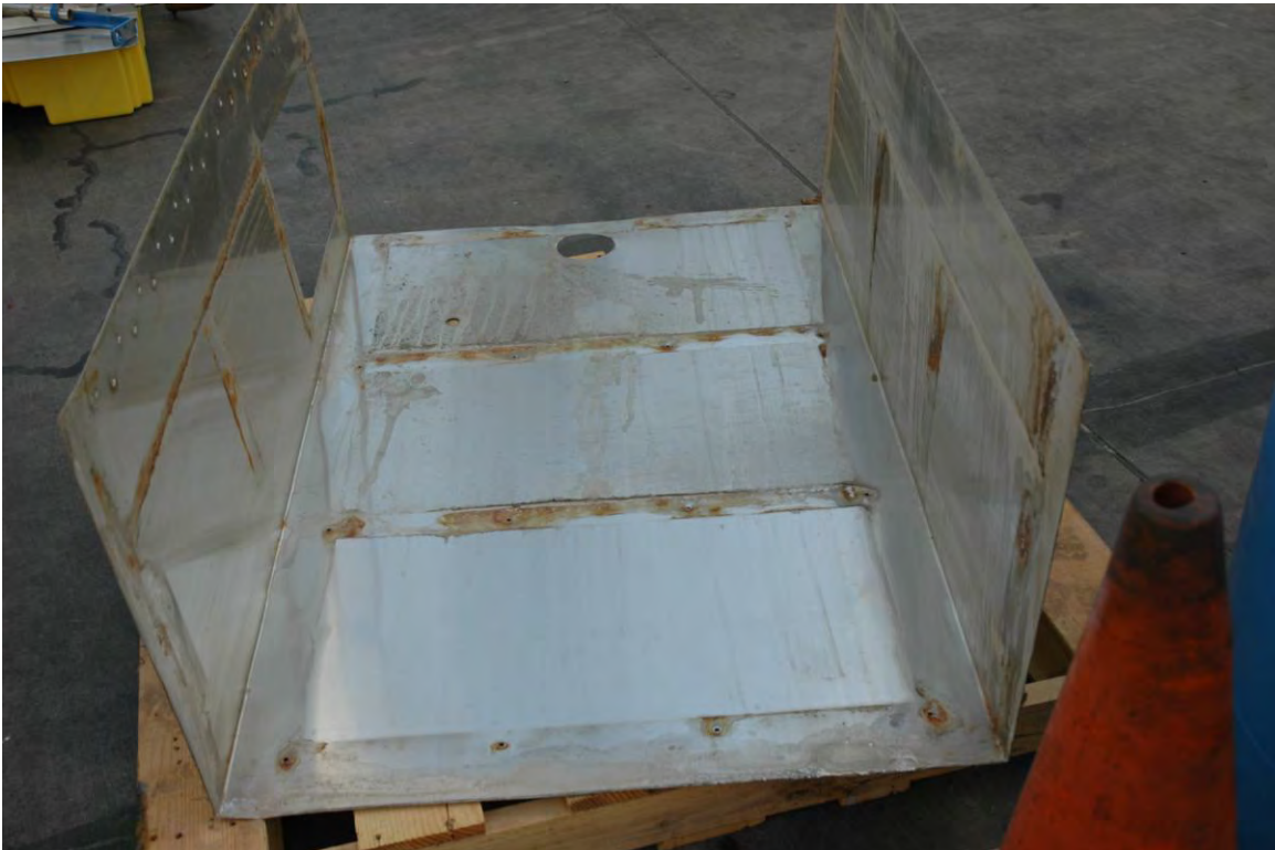
Photo #8: Outer stainless steel covering. Note: rust spots shown
