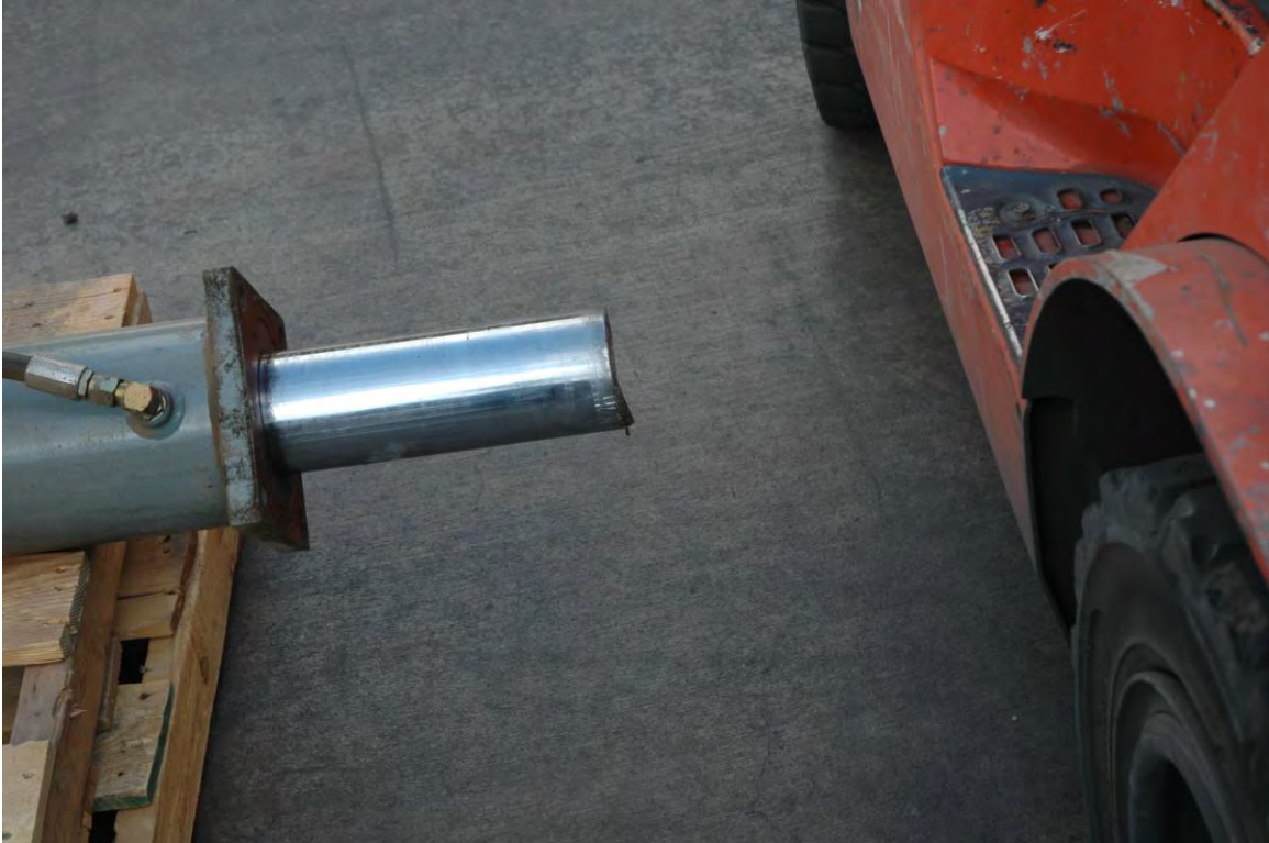
Photo #1: Hydraulic cylinder removed and end with debris cut off for cleaning
