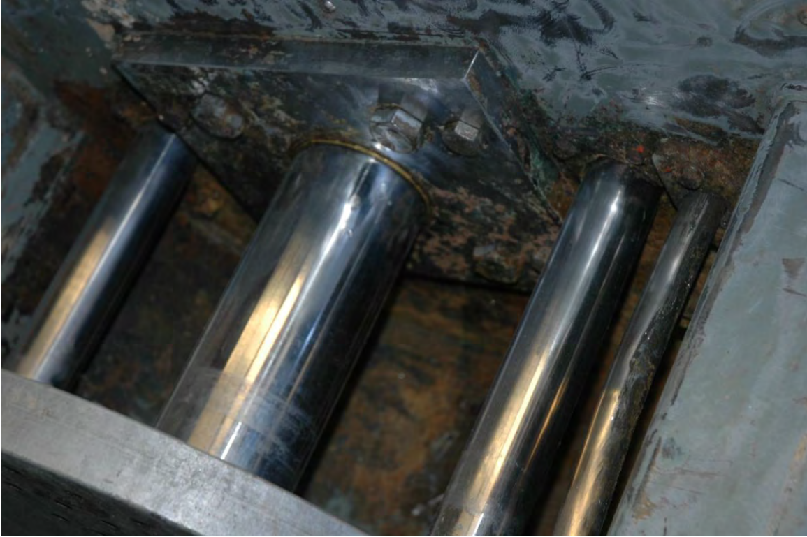
Photo #19: Plunger hydraulic cylinder and related debris
