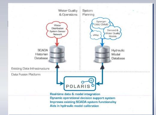
Incorporate continuous online monitoring with the utility's SCADA & hydraulic model. Result: an automated decision supported monitoring and delivery system.
