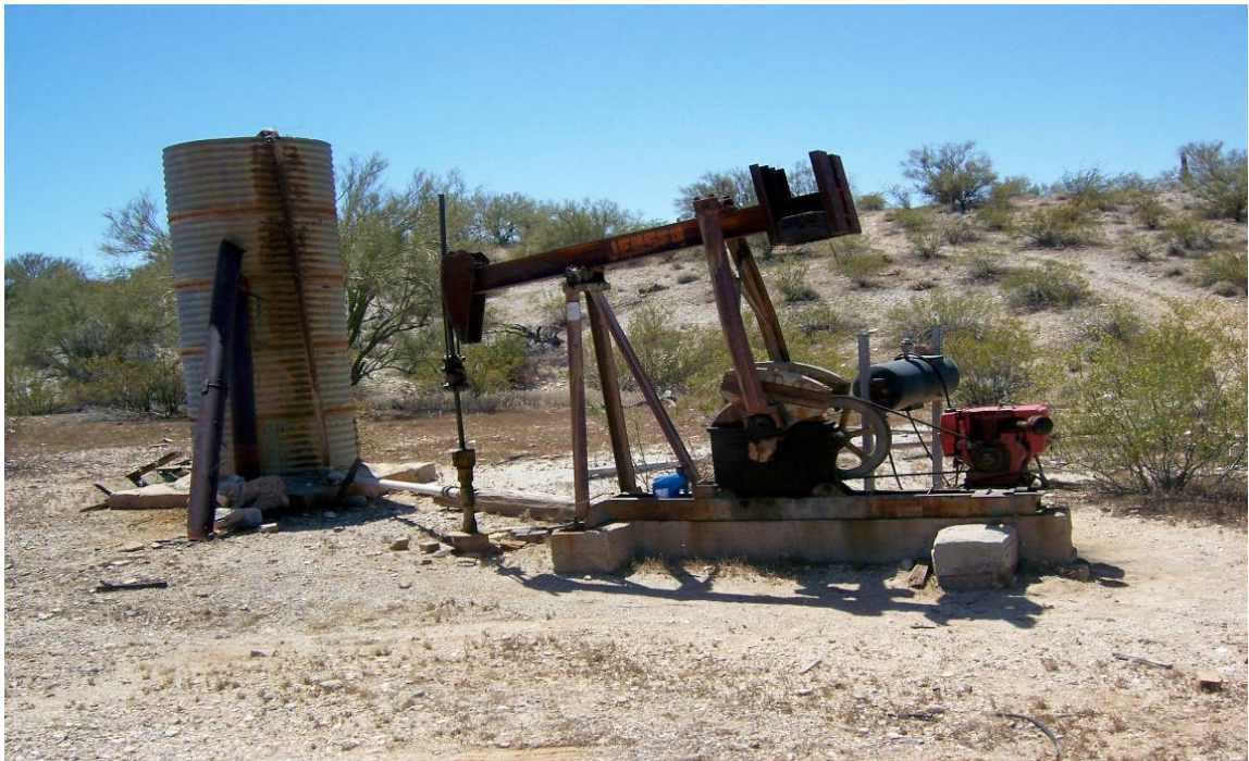
Figure 10 – East Well located in the remote Bullard Wash drainage uses a jack pump to raise groundwater to the surface for stock use. The sample (BWM-99/100) collected from the well met all water quality standards.
