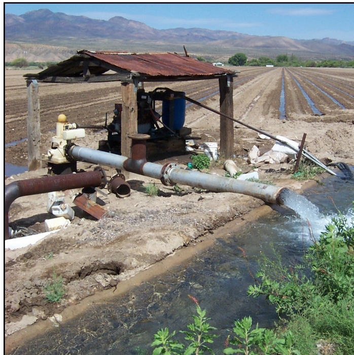
Figure 1 – An irrigation well pumps water from younger alluvium that has been recharged by flow from the Gila River. Emptying into a ditch, the groundwater eventually irrigates a cotton field near the community of Geronimo, just upstream of the San Carlos Apache tribal lands.
