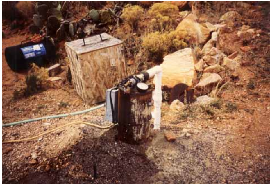
Figure 8. The groundwater sample (HUA-22/23) from this 405-foot deep domestic well in the Music Mountains had water quality exceedances for arsenic, gross alpha, radium 226+228, sulfate and TDS. The well is located in granite, a rock type which is often linked with elevated radiochemistry concentrations, especially in combination with mining operations that expose more rock surface material. 24 The other constituents that exceeded water quality standards, particularly sulfate, are also commonly associated with mining activities. It is not known if any mining had occurred in the vicinity.
