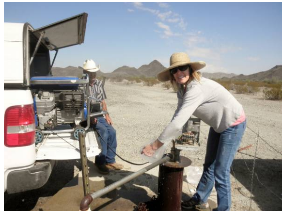
Figure 17 – Many livestock wells in the basin had faucets at the wellhead that made the collection of defensible groundwater samples much easier.
