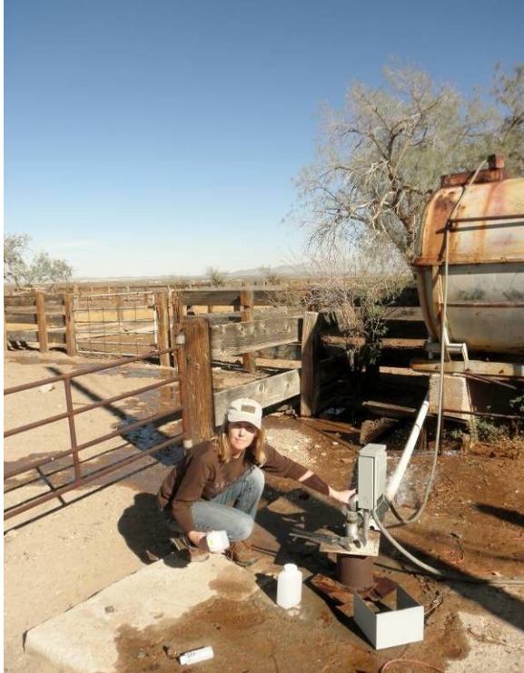
Figure 9 – (RAN-17) ADEQ's Elizabeth Boettcher is shown sampling Swadley Well that provides water for livestock. The sample collected from the well had an arsenic concentration of 0.034 mg/L, one of 35 of 55 sampled sites that exceeded standards.
