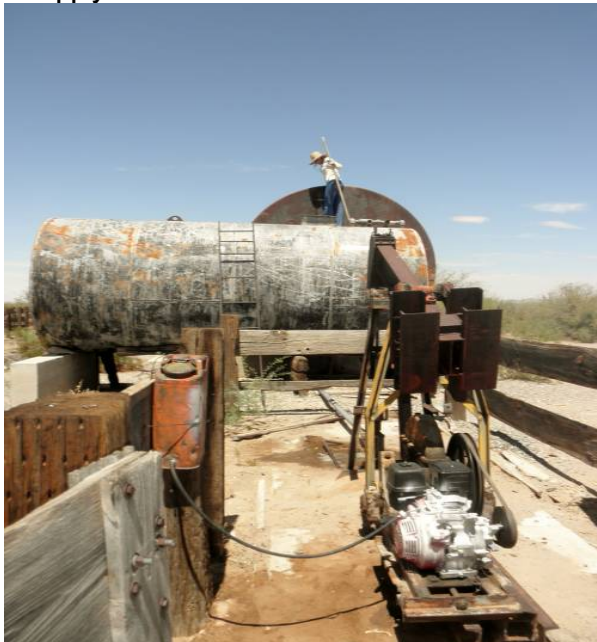
Figure 6 – A vintage jack pump produces water from Chico's Well (RAN-53) to supply livestock. ADEQ's Liz Boettcher can be seen collecting the sample where the pipeline empties into a former underground storage tank.
