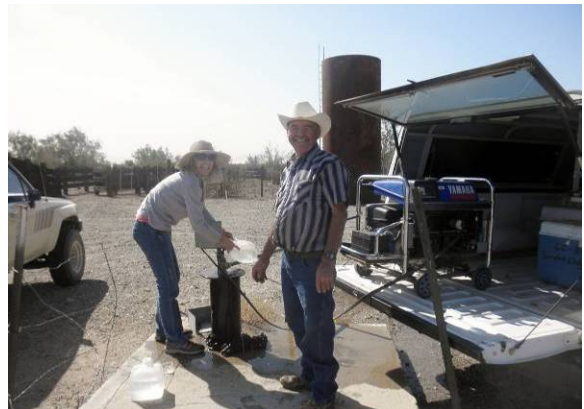
Figure 13 – Ranch foreman Jose Adriano assists ADEQ's Elizabeth Boettcher in collecting a sample from CAP Tank Well (RAN-61). In many areas of the basin, stock wells were the only available sources to collect groundwater samples.
