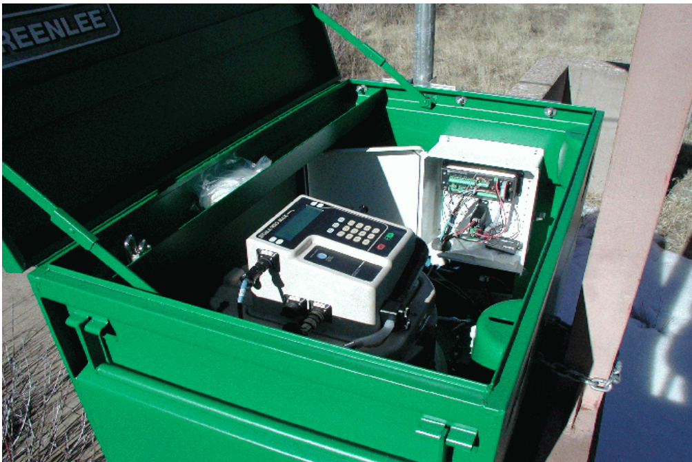
Figure 5. West Fork Black River – ADEQ TTS Station - American Sigma Automatic Sampler with 24 1L Bottles and Campbell Scientific CR10X Data Logger
