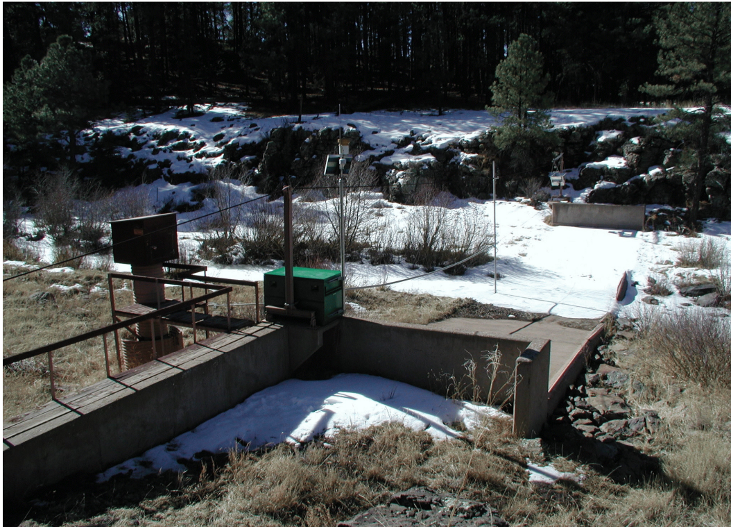
Figure 3. Beaver Creek -USFS Stream gage with Threshold Turbidity Sampling Station
