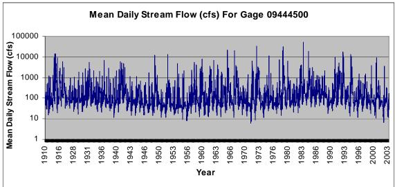
Figure 2-11: USGS Gage 09444500 (San Francisco River at Clifton) Hydrograph.
