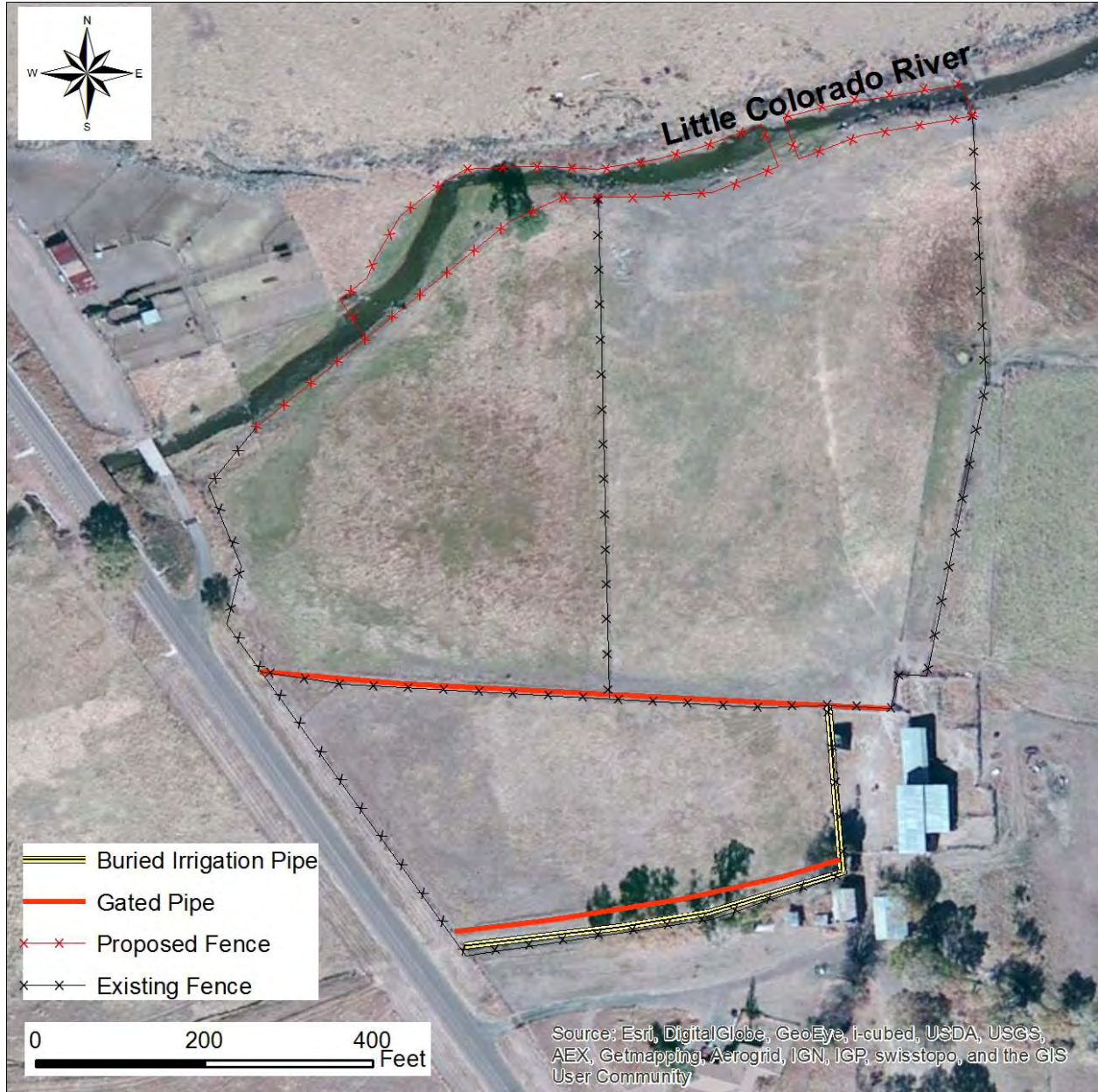
Figure 5. Aerial Photograph with proposed work.
