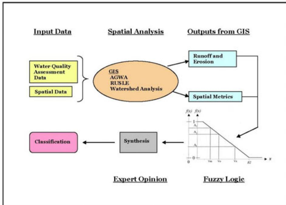
The process was implemented within a GIS interface to create the subwatershed classifications using five primary steps:
