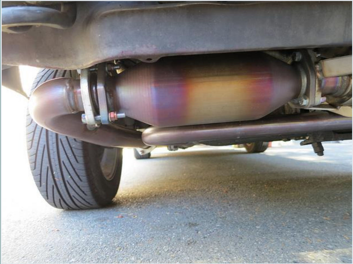
Figure 6. A picture of a catalytic converter on an automobile. Before exiting the tailpipe, the exhaust from the engine passes through the catalytic converter, which changes the molecular structure of the harmful gases and creates harmless gases instead ( explainthatstuff ).
