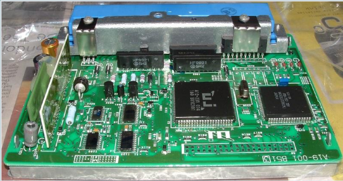
Figure 7. An engine control unit (an automobile's computer) from the late 90s. Public Domain
