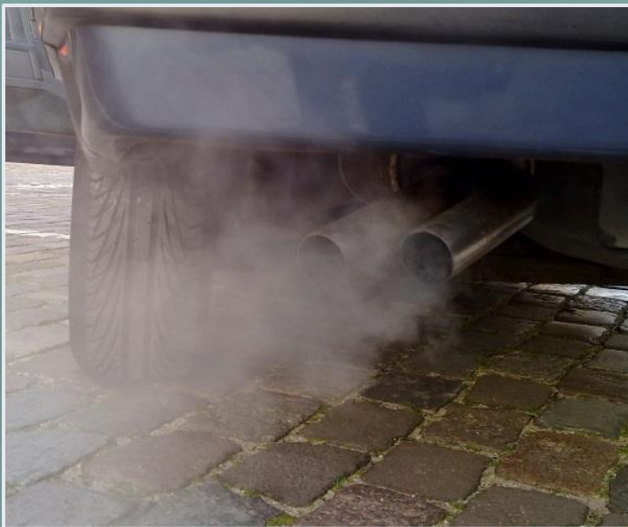
Figure 1. Exhaust from a running car. CO is a small component of vehicle exhaust, which also includes harmless gases such as nitrogen, water vapor, and carbon dioxide and other harmful gases including hydrocarbons and nitrogen oxides ( howstuffworks ).
