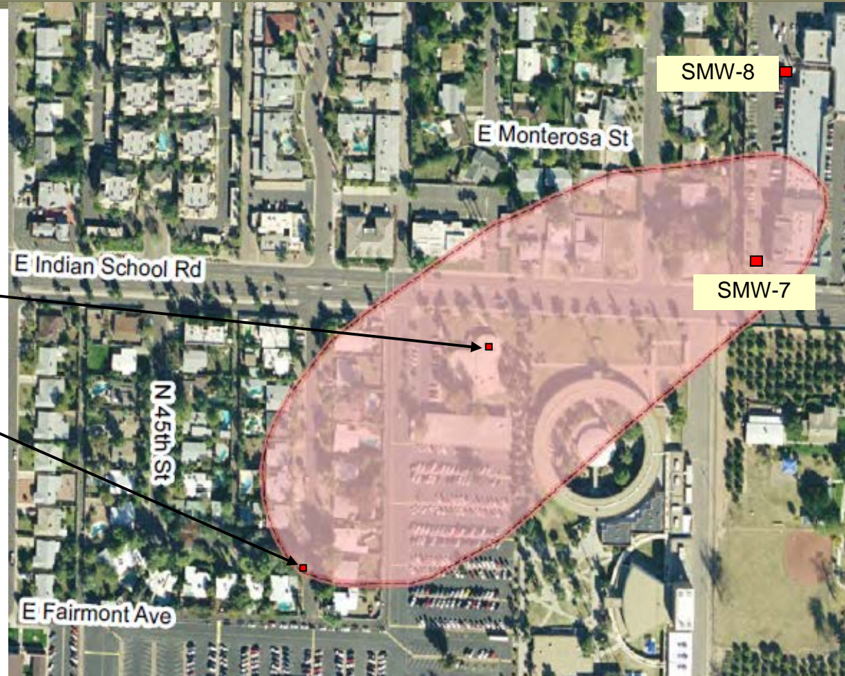
Plume shown is of PCE in groundwater, as of November 2012
