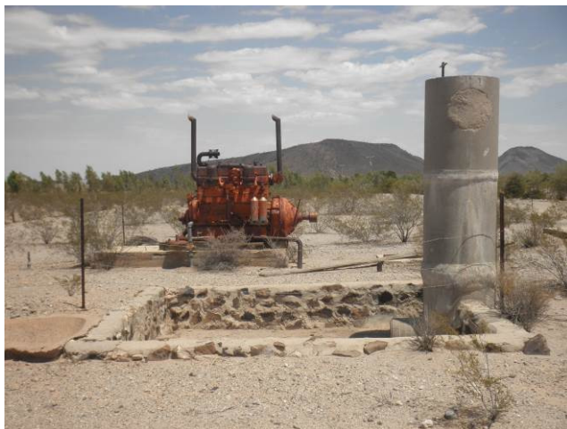
Figure 12 – An irrigation well once powered by a diesel pump sits abandoned in the southeast portion of the basin. The groundwater cone of depression that developed within the HVID severely reduced the amount of water available for agriculture in this area near Mullens Cut. 15
