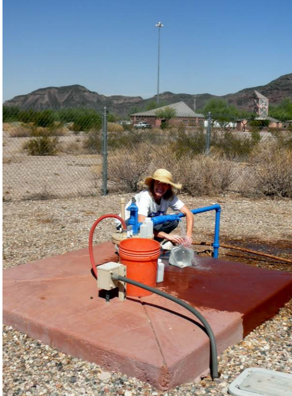
Figure 7 – ADEQ's Elizabeth Boettcher collects a radionuclide sample from the Burnt Mountain Rest Area well located along Interstate 10. A duplicate sample (HAR-5/6) was collected at the site. Laboratory analysis revealed the sample from the 770-foot deep well was soft water with a high pH level (8.89 su) and elevated arsenic concentrations (0.0395 mg/L).
