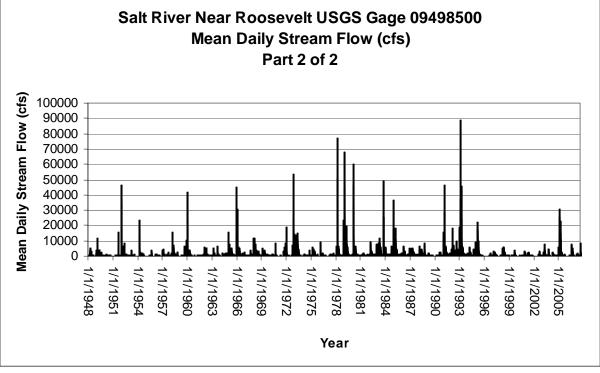
*Figure 2-13: Salt Near Roosevelt USGS Gage 09498500, Mean Daily Stream Flow (cfs) Hydrograph (Part 2 of 2).*
