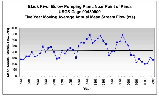
*Figure 2-11: Black River Below Pumping Plant, Near Point of Pines USGS Gage 09489500, Five Year Moving Average Annual Stream Flow (cfs) Hydrograph.*
