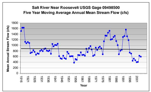
*Figure 2-14: Salt Near Roosevelt USGS Gage 09498500, Five Year Moving Average Annual Stream Flow (cfs) Hydrograph.*
