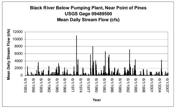
*Figure 2-10: Black River Below Pumping Plant, Near Point of Pines USGS Gage 09489500, Mean Daily Stream Flow (cfs) Hydrograph.*
