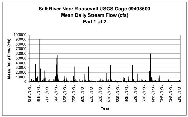
*Figure 2-12: Salt Near Roosevelt USGS Gage 09498500, Mean Daily Stream Flow (cfs) Hydrograph (Part 1 of 2).*
