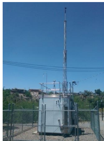
Hayden Old Jail shelter, PM inlet and meteorological tower – 05/2014
