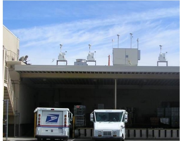
Particulate and meteorological monitors on roof of Nogales Post Office – 04/2013
